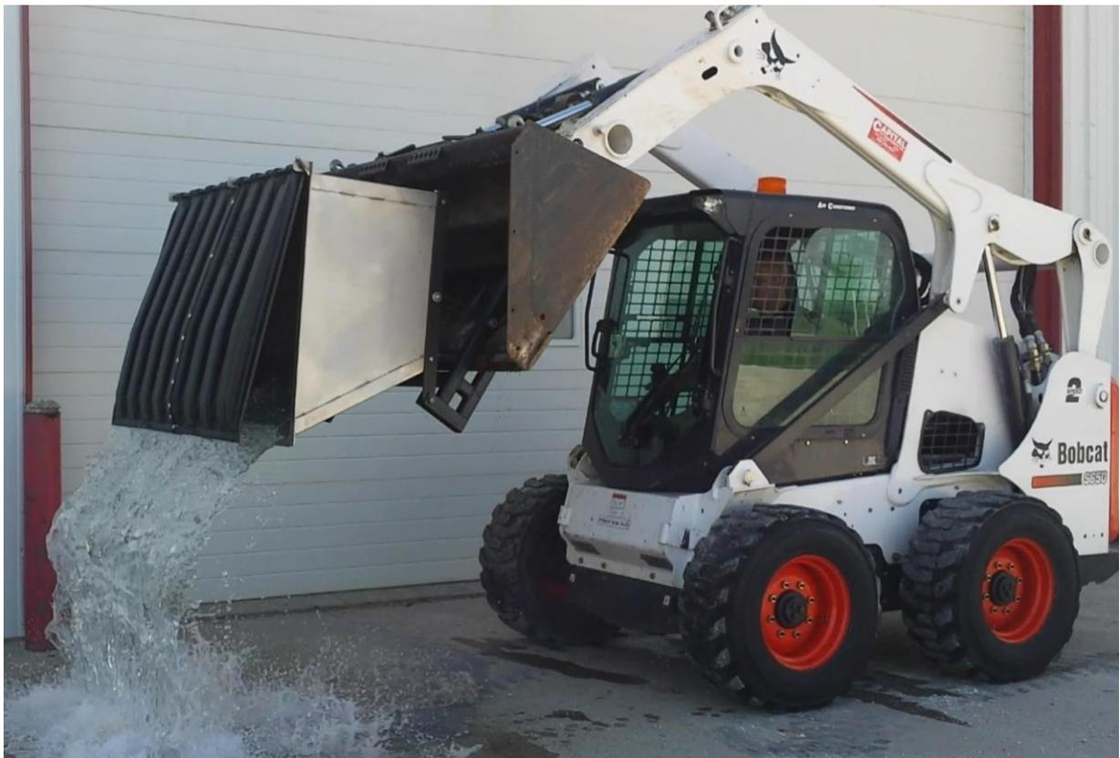
7. Once the Chuck-It Bucket is completely emptied, tip the loader bucket back into a level position and lower. The Chuck-It Bucket will return to its resting position on its own.
