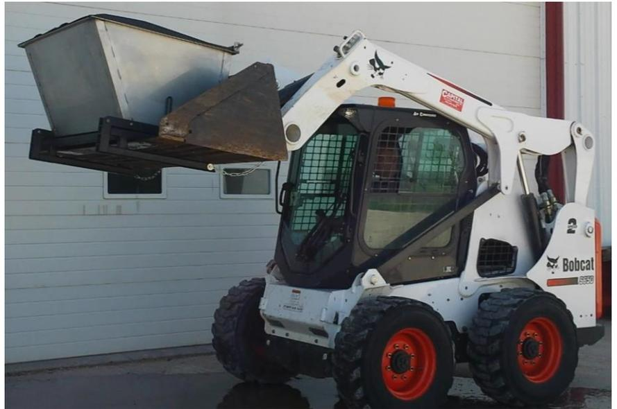
8. Drive back to the Chuck-It Bucket's original location. Un-hook the chains from the back of the loader bucket. Lower the bucket onto the ground and back away. Hook the rubber straps back on the lid to keep it from blowing open.
