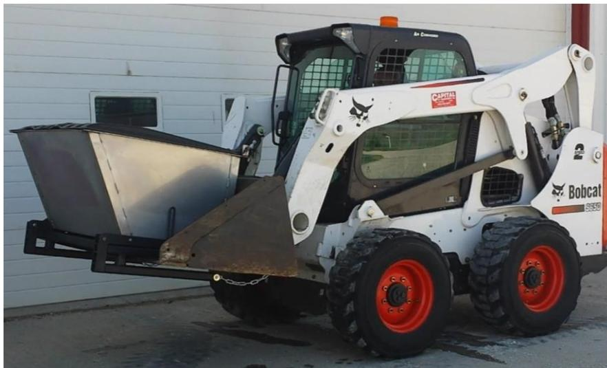
5. Once at destination, unlatch both rubber straps on the lid for dumping. If outside temperature is below freezing point, using a large propane torch, warm the stainless steel portion of the Chuck-It Bucket, making sure all surface is covered, but not getting too close to the plastic lid.
