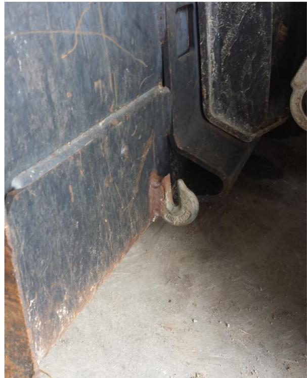
2. Drive up to the Chuck-It Bucket, lowering and leveling the loader bucket so that the cutting edge will slide into the open slot of the Chuck-It Bucket. Drive until the cutting edge stops below. Raise the loader bucket slightly so that the Chuck-It Bucket is resting on the loader bucket.
