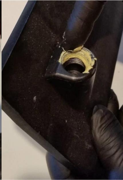
**10.** To install drinking nipples and hose barb fixture, smear small amount of Pipe Thread Sealant in the first few threads on each opening of the SnoutSpout.
