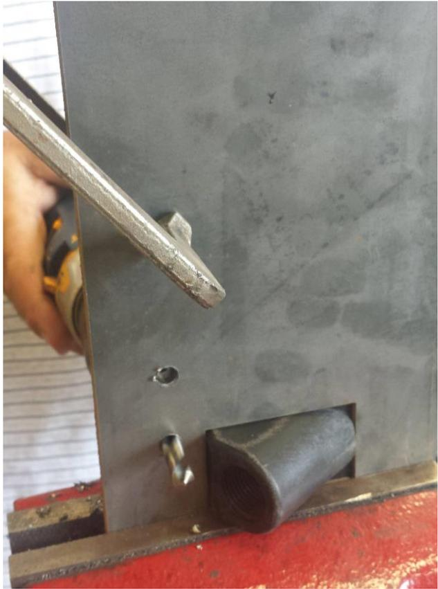
8. Find desired location for top bolt and drill through top bar or angle iron. Place SnoutSpout in desired location and drill through top of SnoutSpout. Secure SnoutSpout with bolt.
