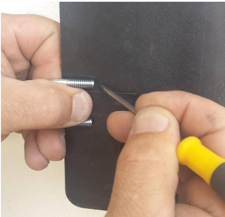
**4.** With the awl, mark area where you intend to drill holes for U-Bolt, centering the U-Bolt where the bar crosses the SnoutSpout mounting plate.
