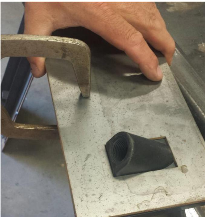
**6.** Place template on SnoutSpout and clamp securely. The template fits on the flat side of the SnoutSpout.
